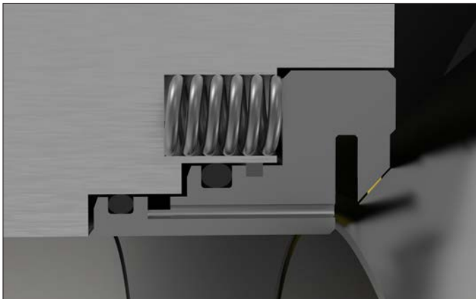
Figure-3 - Metal to metal hoop design*
